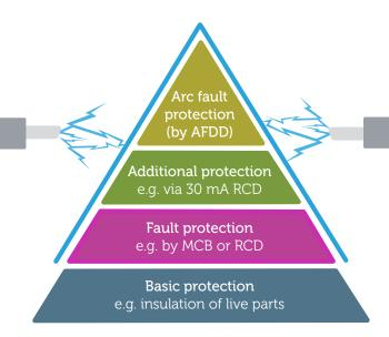
AFDDs provide additional protection that is not offered by MCBs and RCDs. AFDDs detect low level hazardous arcing that MCBs, Fuses & RCDs are not able to detect.
